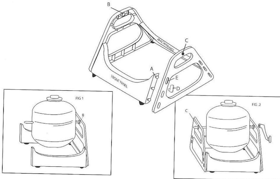
1. Connect the front and back panels to one of the side panels by pressing the joining lugs "A" into the corresponding holes and slide into position.
