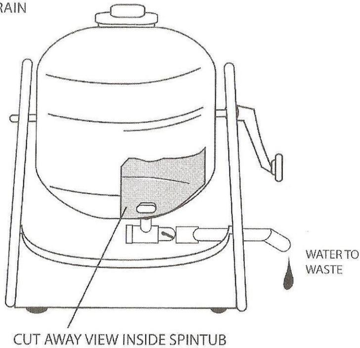
1. The water release valve is situated underneath the tub and slightly to the right.
